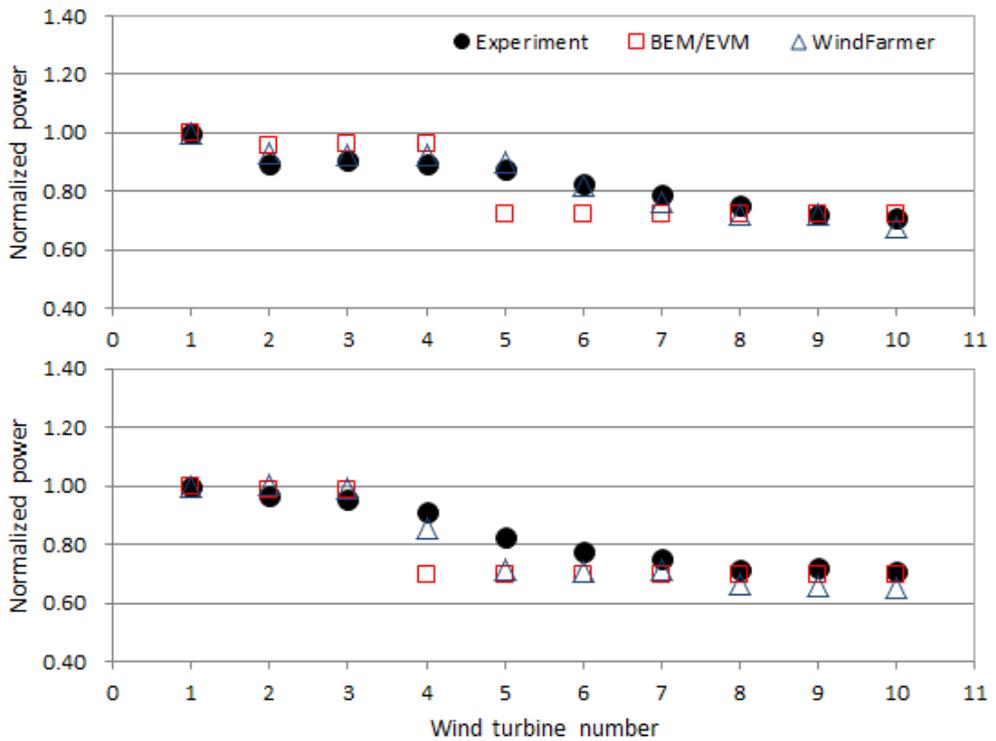
Fig. 4. Normalized power at Horns Rev offshore wind farm of the ER+10° case(top) and ER+15° case(bottom).
