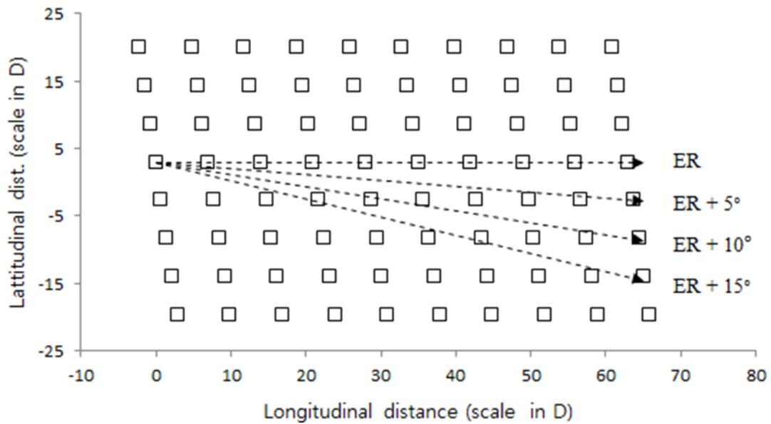
Fig. 2. Layout of the Horns Rev offshore wind farm
