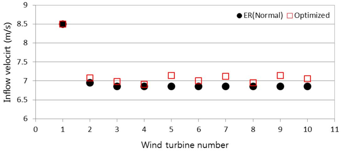
Fig. 9. Averaged inflow velocity on the rotor plane in optimized condition.
