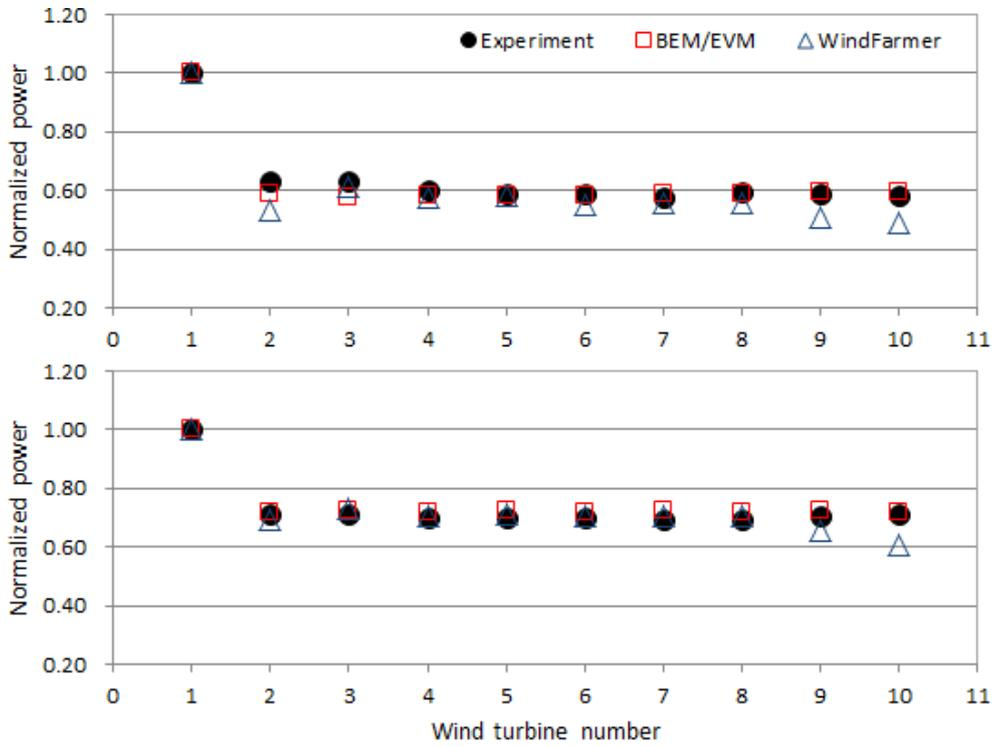
Fig. 3. Normalized power at Horns Rev offshore wind farm of the ER case(top) and ER+5° case(bottom).
