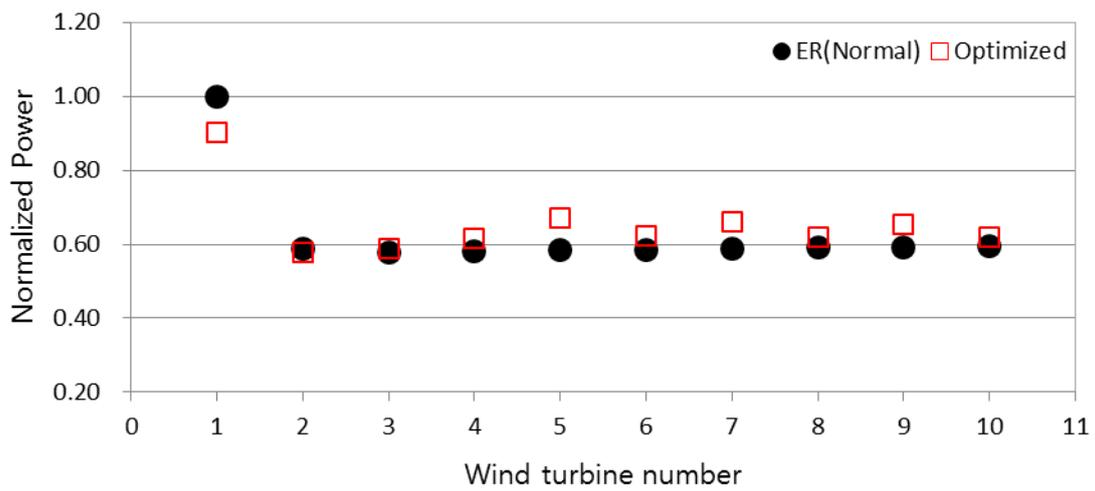
Fig. 8. Optimized result of the normalized power of each wind turbine compared to the normal condition.
