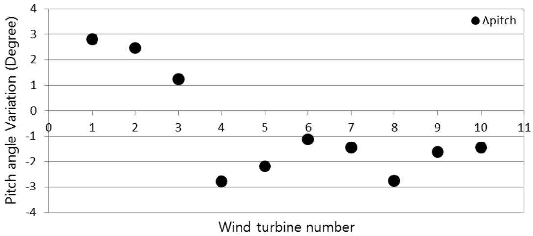
Fig. 10. Pitch variation of each turbine optimizing the wind farm power output.
