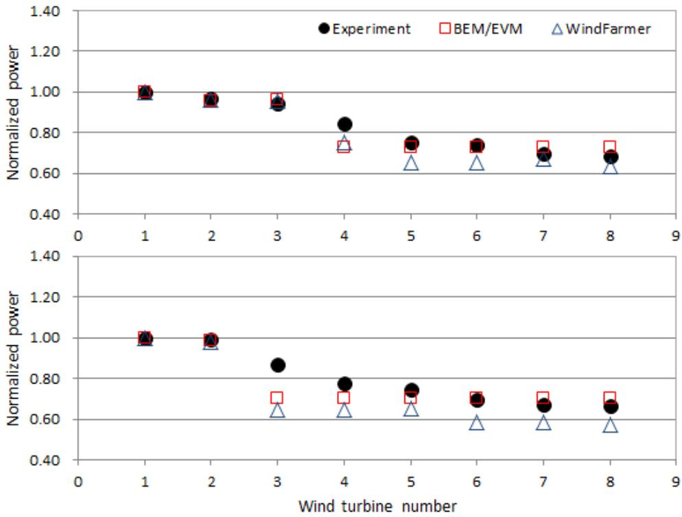
Fig. 7. Normalized power at Nysted offshore wind farm of the ER-10° case(top) and ER-15° case(bottom).
