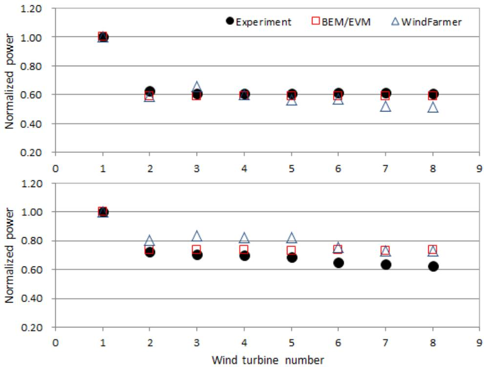
Fig. 6. Normalized power at Nysted offshore wind farm of the ER case(top) and ER-5° case(bottom).
